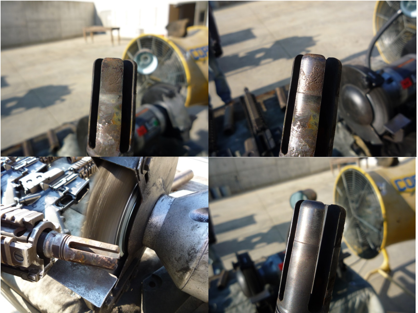
Figure 13 – Flash Hider Deposits and Cleaning
