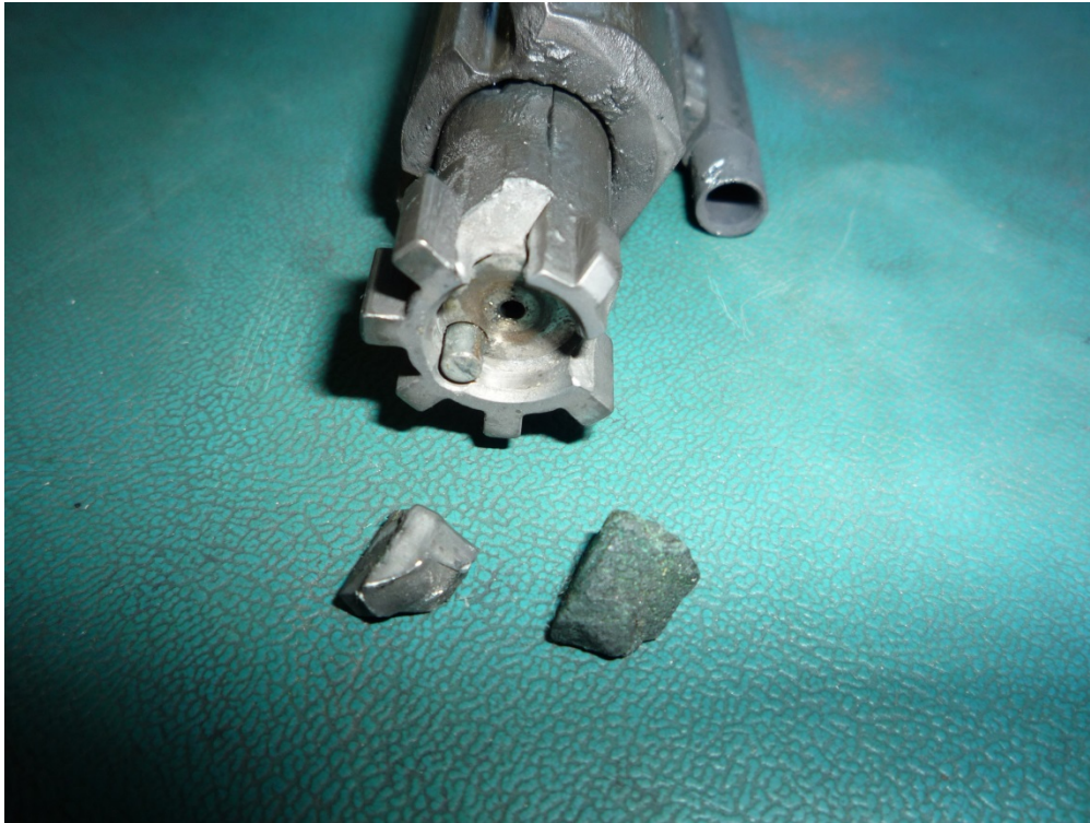
Figure 11 – Broken Bolt Lugs
